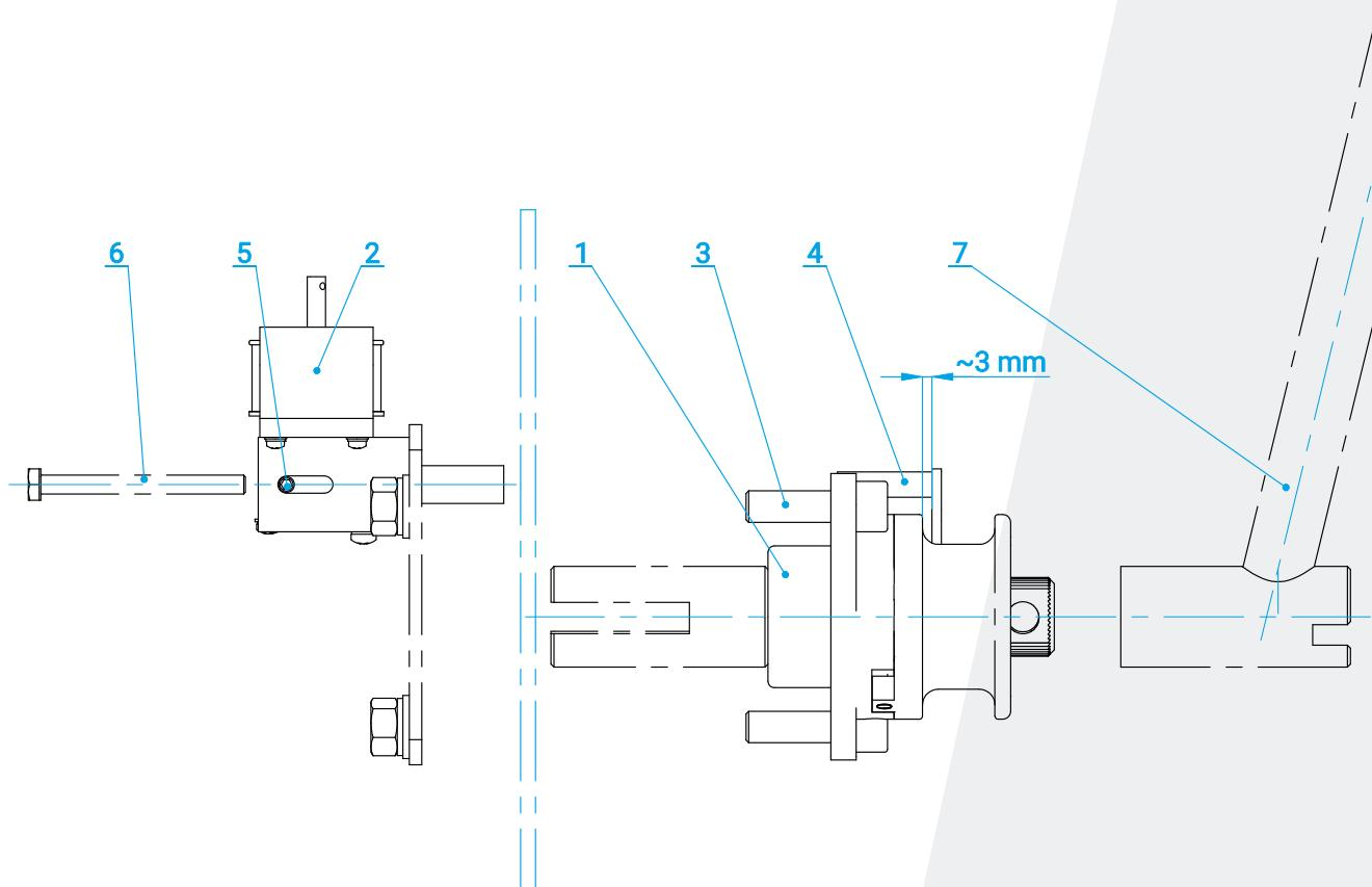
After checking the correctness of the operation of the drive interlock, the M6x65 bolt must be locked with two M5x12 Allen screws [5].
